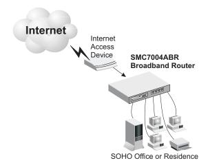
Figure 2. Connecting the Barricade Router
